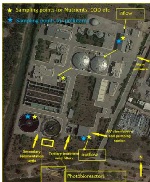
Fig. 1. The microalgae bioreactors system at Thrasio WWTP.
